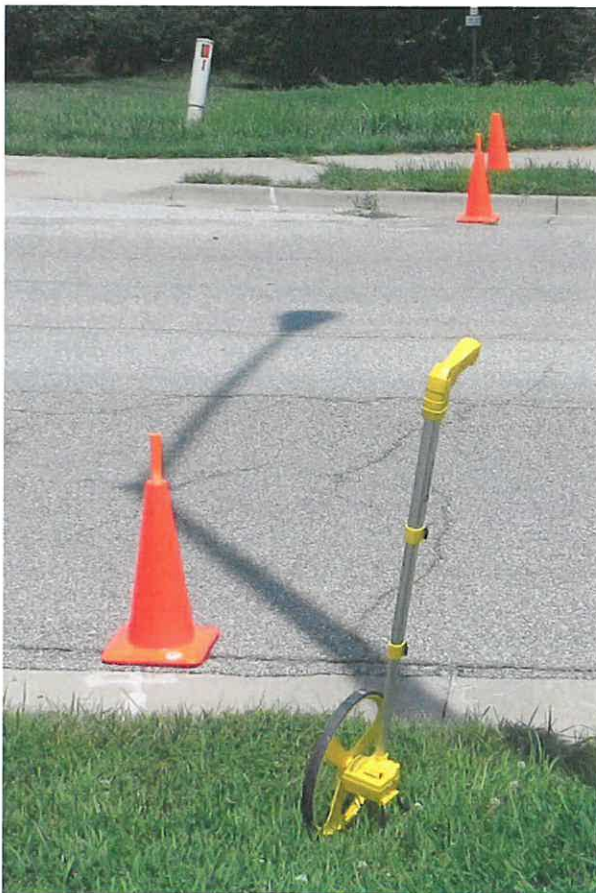
Figure 34 - Stopping Sight Distance 2-Foot Object Height Markers and Rolling Wheel
